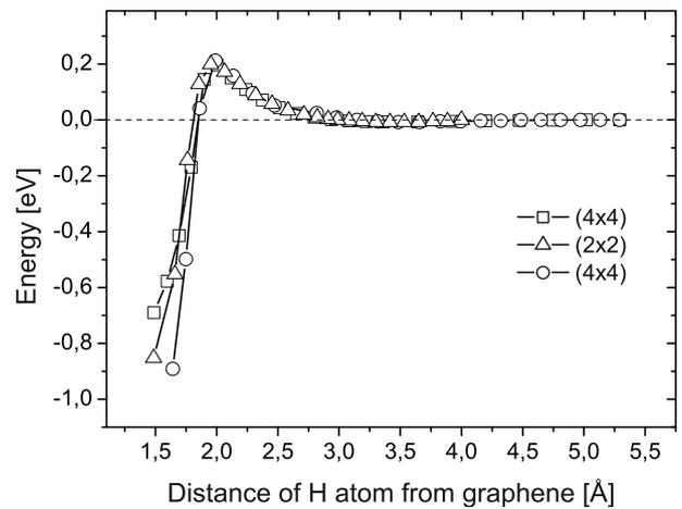
**Fig. 3.** Comparison of energy curves for adsorption of an H atom onto graphene: squares, optimization of the sole adsorbent C atom within a  $(4 \times 4)$  cell; triangles and circles, full NEB relaxation of  $(2 \times 2)$  and  $(4 \times 4)$  cells, respectively.
