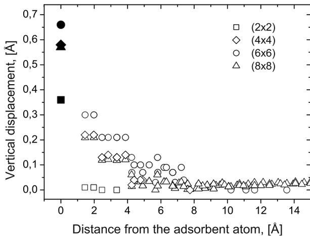
**Fig. 2.** Vertical displacements of atoms versus in-plane distance from the adsorbent carbon atom. Squares, diamonds, circles and triangles stand for  $(2 \times 2)$ ,  $(4 \times 4)$ ,  $(6 \times 6)$  and  $(8 \times 8)$  supercells, respectively. The position of the adsorbent atom for each supercell is marked by a closed symbol.
