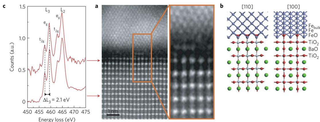
**Figure 4 | Interface structure analysis.** **a**, Atomically resolved HAADF image of the Fe/BTO interface of the Fe/BTO(50 nm)/LSMO(30 nm) //NGO(001) heterostructure. **b**, Structural model of the type II interface, that is,  $-\text{Fe}-\text{FeO}-\text{TiO}_2-\text{BaTiO}_3$ . **c**, Ti  $L_{2,3}$ -edge spectra acquired on  $\text{TiO}_2$  columns located in the BTO layer (blue line) and next to the Fe layer (red line).
